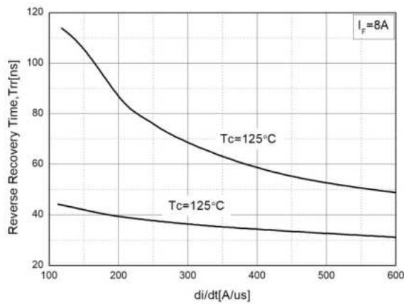
Fig. 4. Typical Reverse Recovery Current vs.  $\text{di}/\text{dt}$
