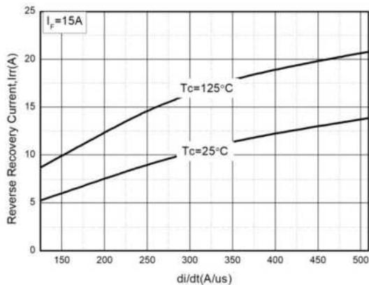
Fig. 4. Typical Reverse Recovery Current vs.  $di/dt$
