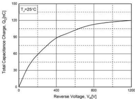
Fig. 4. Typical Characteristics:  $V_R$  vs. C (pF)
