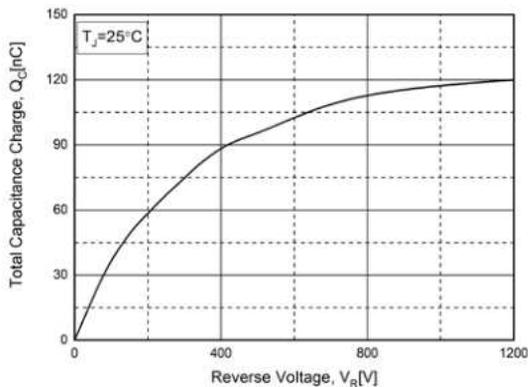
Fig. 4. Typical Characteristics:  $V_R$  vs. C(pF)
