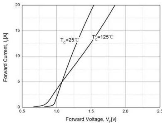
Fig. 2. Typical Characteristics:  $V_F$  vs.  $I_F$
