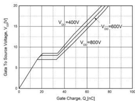
Fig. 8. Characteristics vs. Drain-to-Source Voltage
